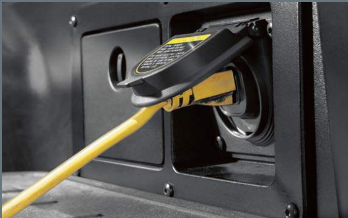
3 AVAILABLE 115V/400W DECK-MOUNTED AC POWER OUTLET
