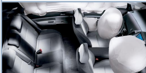
Driver and front passenger dual-stage airbags 1 and available front seat-mounted side and front and rear side curtain airbags. 1
