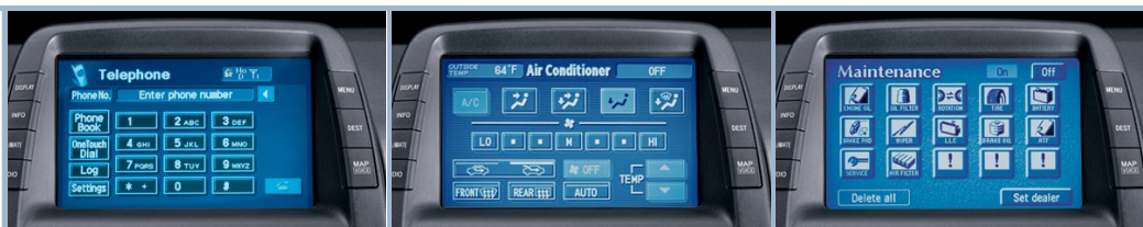
Multi-information display with hands-free phone screen with Bluetooth™ technology/air conditioning/maintenance screen.
