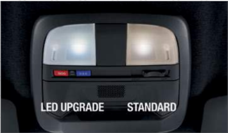
LED Upgrade. The LED Upgrade offers brighter, whiter and crisper interior lighting than the standard equipment lighting.
