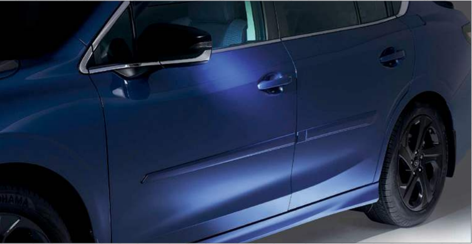
Auto-Dimming Exterior Mirror with Approach Light Make it easier—and safer—to come and go with the accessory Auto-Dimming Exterior Mirrors with Approach Light. 1 When the doors are opened or unlocked with the key fob, LED lights on the side-view mirrors will help illuminate the way, casting light on all four doors and the ground near the vehicle. They can also help reduce headlight glare in traffic. When the Auto-Dimming Interior Mirror detects excessive light from the rear of the vehicle, the side-view mirrors automatically dim, helping to keep the glare out of your eyes. The brighter the light, the dimmer the mirrors and the better you'll be able to see.
