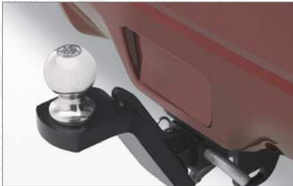
Trailer Hitch. Rated at 200 lbs tongue weight with 1,500 lbs of towing capacity. Engineered to the same rigorous standards as the rest of the Crosstrek. Hitch ball not included. Trailer brakes may be required. Excludes Hybrid models.
