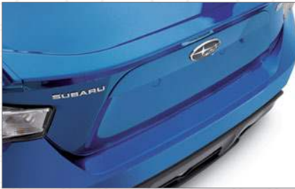
Rear Bumper Appliqué. Clear, scratch-resistant vinyl film helps to protect bumper upper surface and leading edge. Includes a discreet pearl-colored Subaru logo.
