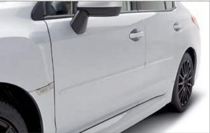
Body Side Moldings. Color-matched moldings help protect the vehicle's doors from parking lot dings while attractively blending with the lines of the car.
