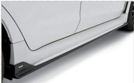
STI Side Underspoiler. Continue the mean ground-hugging attitude down the rocker panels of the WRX or STI. Kit includes left and right side underspoilers.
