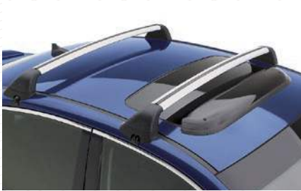
Crossbar Set Fixed — Sedan. May be used in conjunction with most Genuine Subaru roof attachments and carriers. Additional mounting clamps required.
