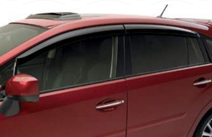
Side Window Visors. Designed to let the fresh air in while helping to keep the rain out of the vehicle. Black acrylic plastic construction is designed specifically for an exact fit on the Impreza models. May not be legal in all states. Please check the laws of your state.
