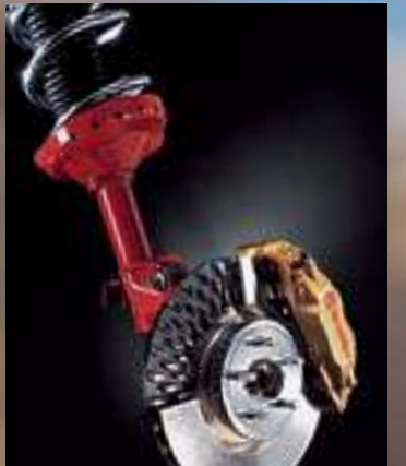
The rally-inspired inverted struts of the WRX STi increase lateral rigidity, improving performance under hard cornering.
