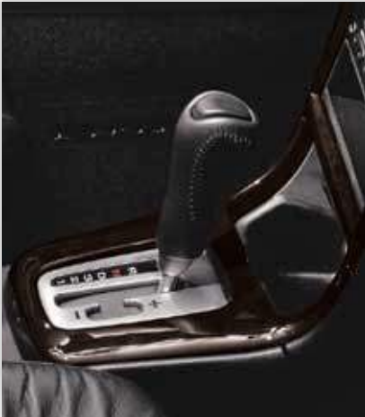
SPORTSHIFT: Legacy 2.5 GT models equipped with the optional 4-speed automatic transmission feature SPORTSHIFT that allows easy manual shifting, if desired.
