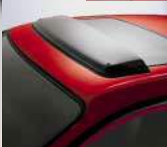
Accessory moonroof air deflector helps reduce wind noise and cut sun glare.
