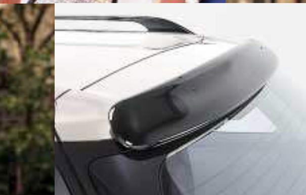
Accessory rear window dust deflector helps keep back window clear of dust for better vision.
