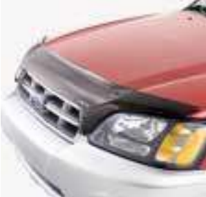
Hood protector. Durable acrylic plastic wrap-around design helps protect the Baja hood from stone chips and bugs.
