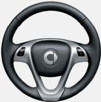
3-spoke leather sport steering wheel with cruise control or paddles for manual battery recuperation: Energy at your fingertips. Literally. Using the steering wheel paddle shifters helps your smart increase the battery's range, giving you more juice for your journey.
