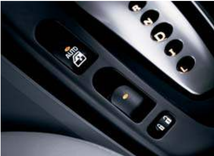
Power windows. The driver express-down feature allows one-touch ease, while the rear window lock helps control access from the back seat.
