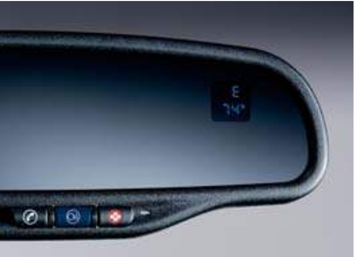
Auto-dimming interior rearview mirror. In addition to dimming for better nighttime visibility, this electrochromatic mirror displays temperature and compass direction.
