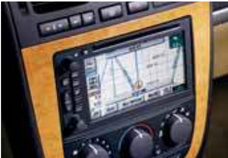
GPS navigation radio. Uses GPS and a mapping DVD to visually and audibly tell you how to get from here to there. A CD player and radio are also integrated into the system.
