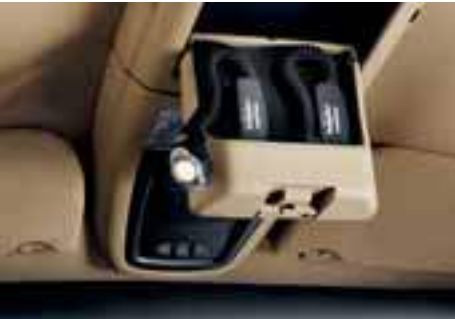
Overhead bin inserts. You can add up to three bins to the overhead rail storage system. Available inserts include flashlights, CD/DVD case, first-aid kit, and more.
