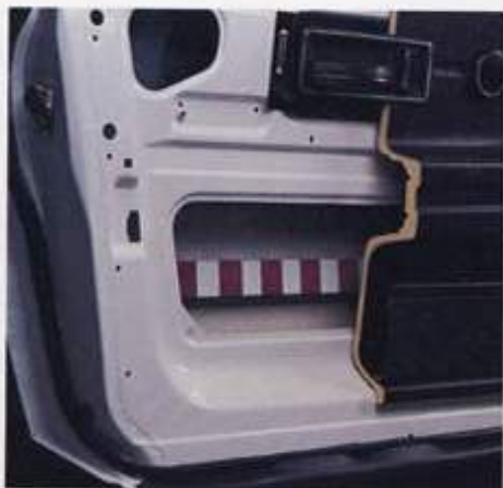
A steel safety cage surrounds passengers in a Saab 900.
