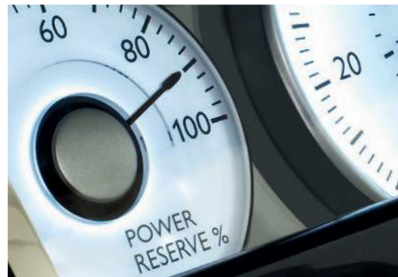
All Rolls-Royce motor cars feature a Power Reserve dial on their fascia rather than a rev counter. The analogue dial informs the driver how much power they are using and how much they have left at their disposal.
