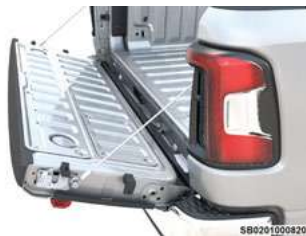
Tailgate Only Supported By Cables
