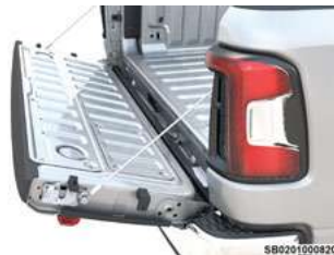
Tailgate Only Supported By Cables
