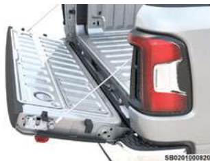
Tailgate Only Supported By Cables
