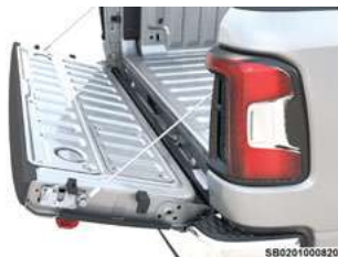
Tailgate Only Supported By Cables
