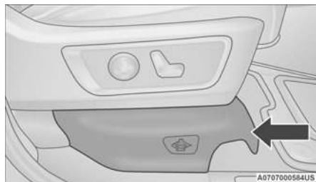
Pull Jack Access Cover From Front
