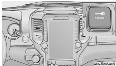
Power Outlet — Top Of Center Stack
