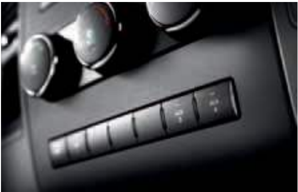
BUILT-IN UPFITTER SWITCHES.
