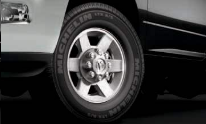
17-inch Polished Forged Aluminum Wheel (Standard on 2500/3500 SRW Big Horn/Lone Star, Available on SLT, Outdoorsman)
