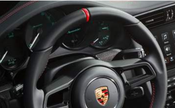
Steering wheel rim with top centre marking in red
