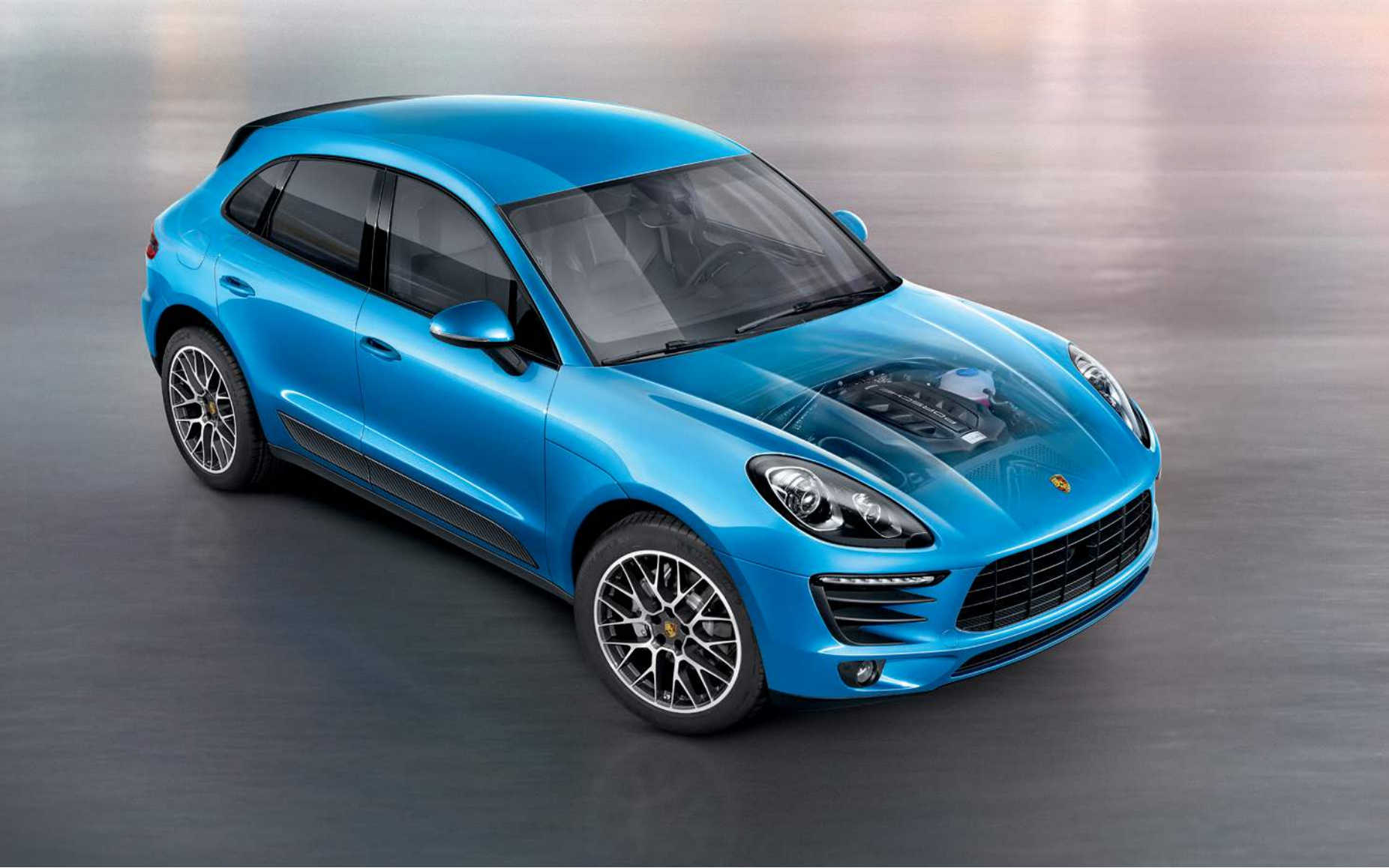
3.0-liter twin-turbo V6 engine
