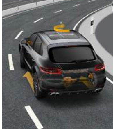
Porsche Torque Vectoring Plus (PTV Plus)
