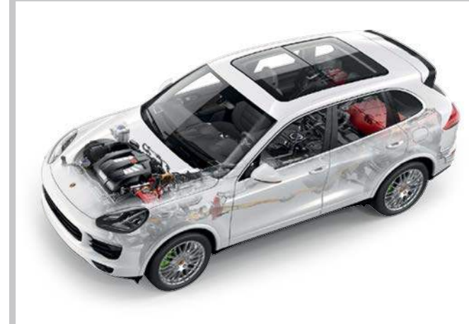
Drivetrain of the Cayenne S E-Hybrid
