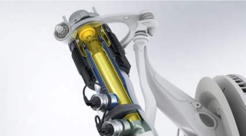
Adaptive air suspension with three-chamber technology
