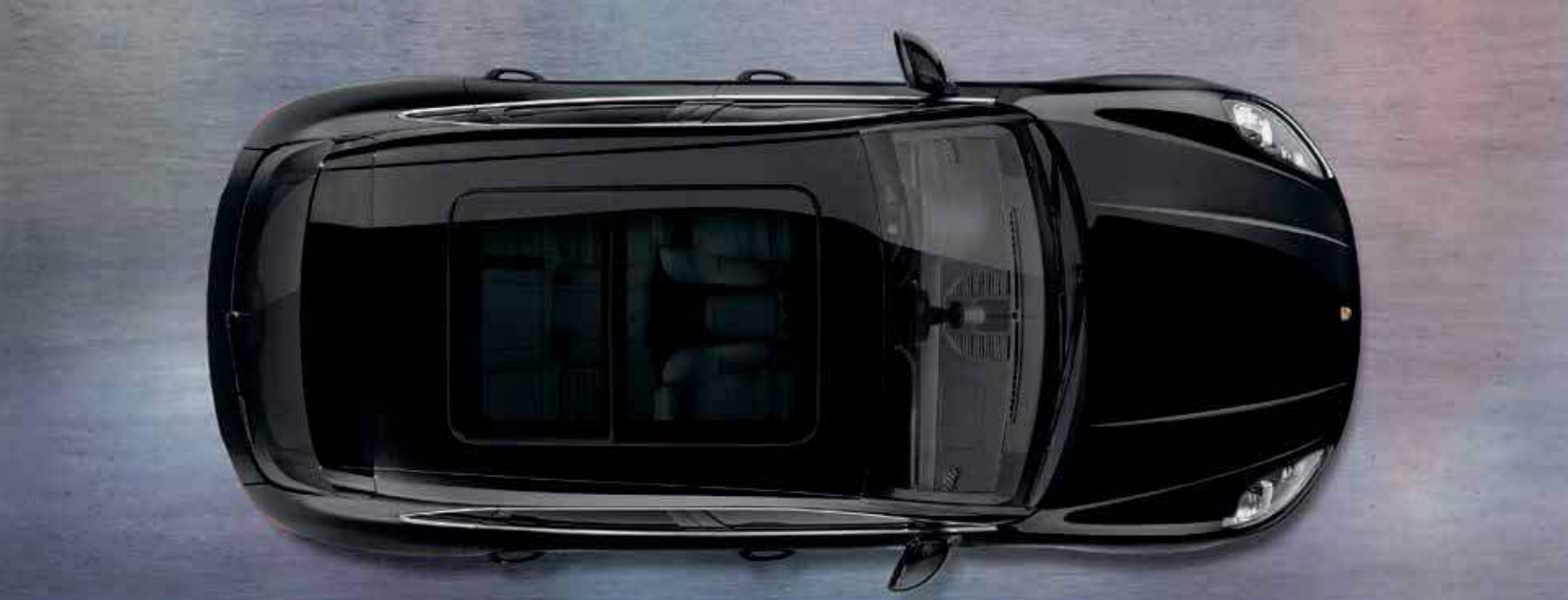
Panoramic roof system
