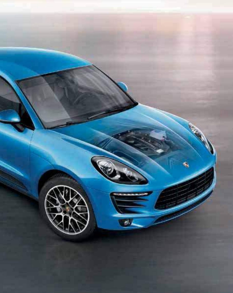
3.0-liter, twin-turbo V6 engine
