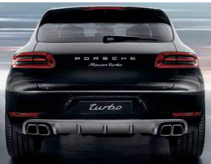
Stainless steel skid plate (rear)
