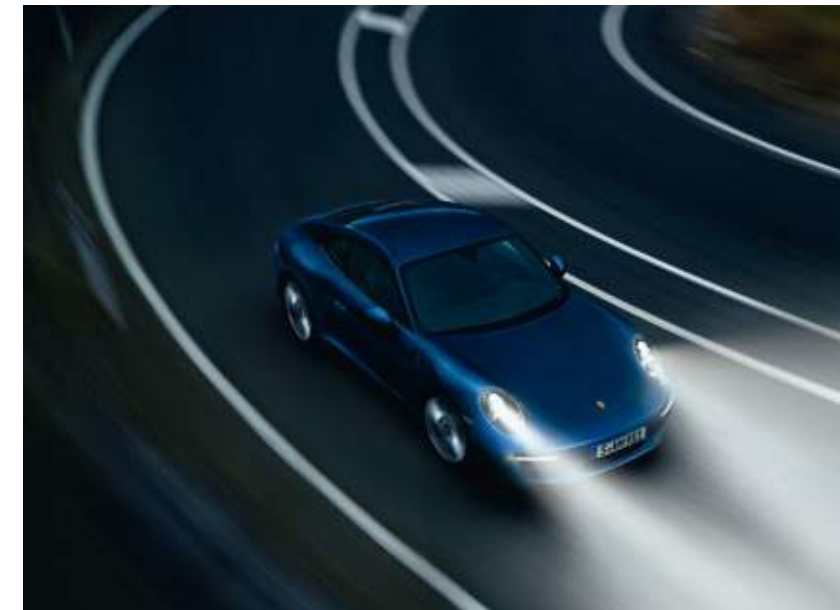
Porsche Dynamic Light System (PDLS) cornering lights
