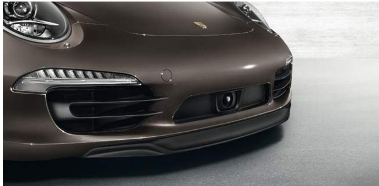
Radar sensor of adaptive cruise control
