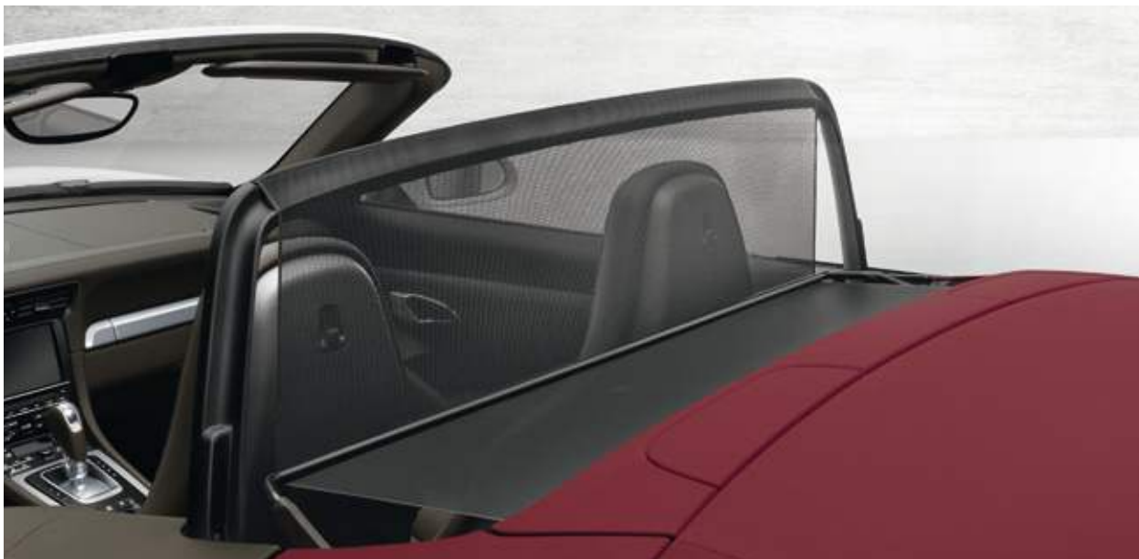
Electrically powered wind deflector
