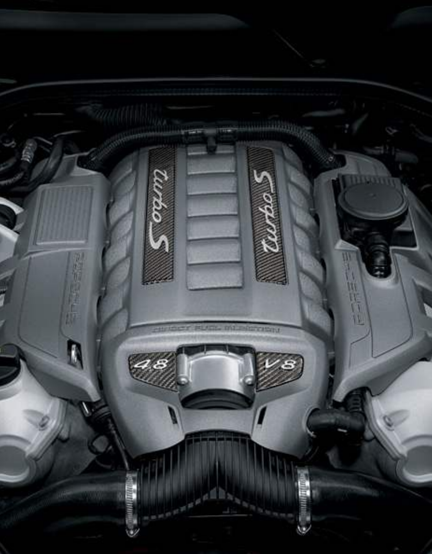
4.8-liter twin turbo V8 engine
