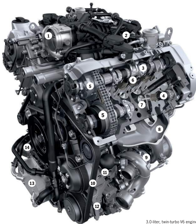
3.0-liter, twin-turbo V6 engine
