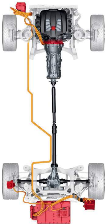
Hybrid components of the Panamera S E-Hybrid
