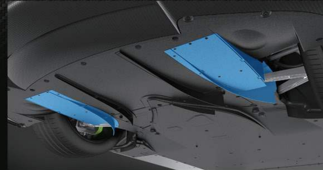
Diffusers in the underfloor
