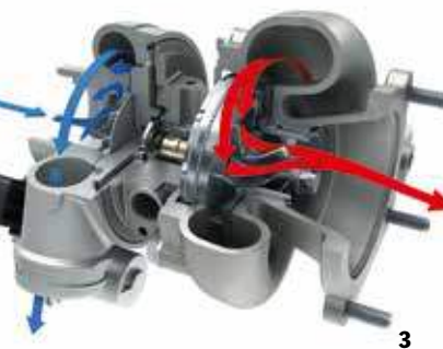
1 Vanes closed | 2 Vanes open | 3 Variable Turbine Geometry (VTG)
