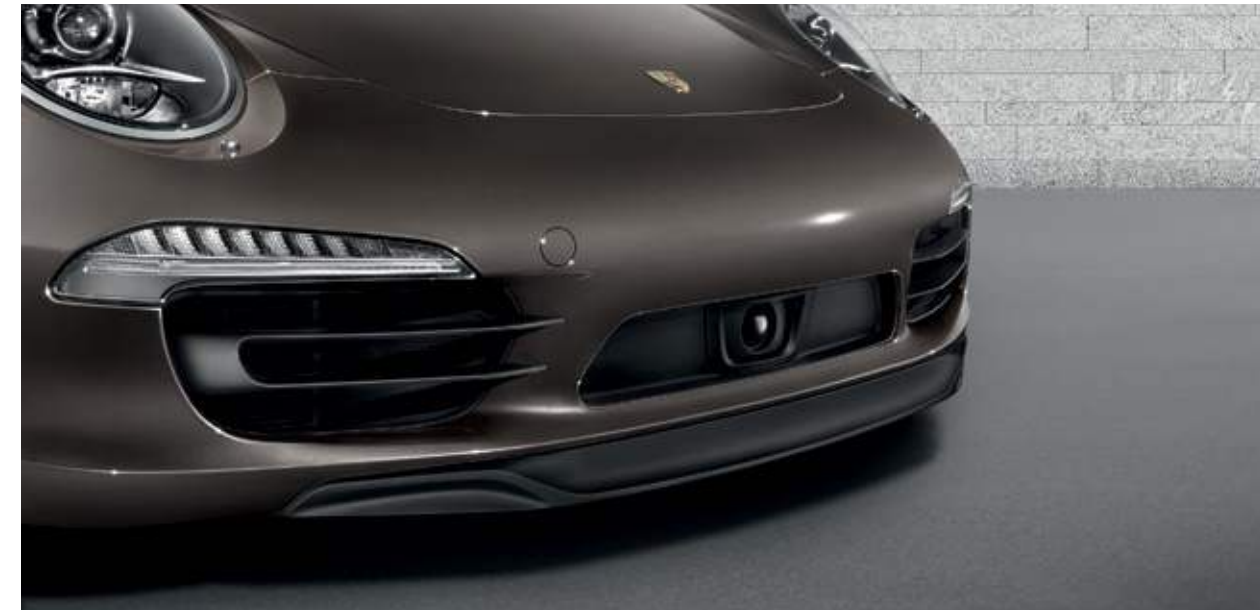
Radar sensor of adaptive cruise control
