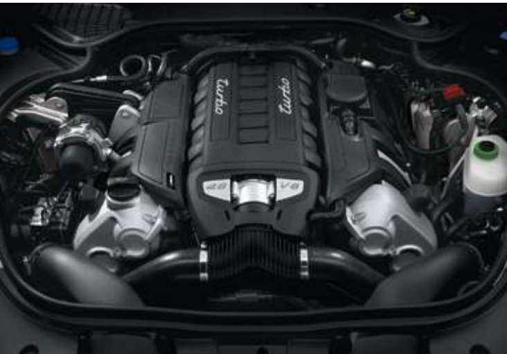
The V8 twin-turbo engine in the Panamera Turbo
