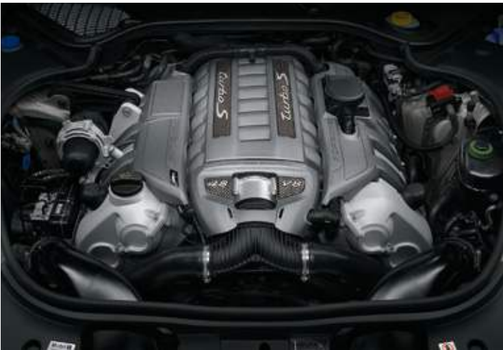
The V8 twin-turbo engine in the Panamera Turbo S
