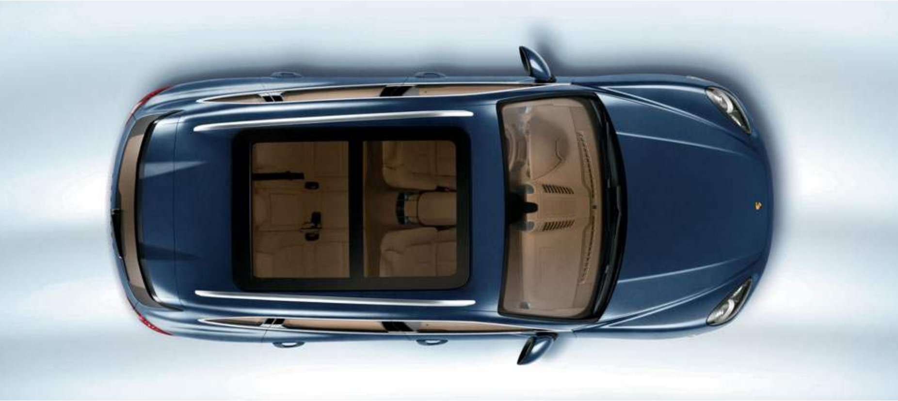
Panoramic roof system
