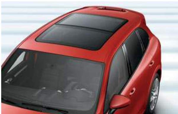
Panoramic roof system
