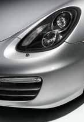
Bi-Xenon™ headlights including Porsche Dynamic Light System (PDLS)
