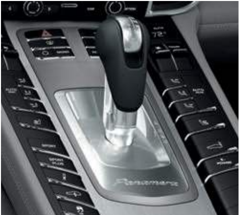
Eight-speed Tiptronic S gearbox
