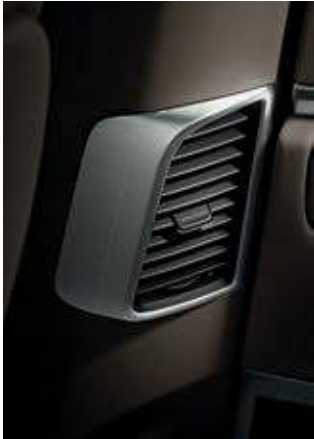
Air-vent in rear
