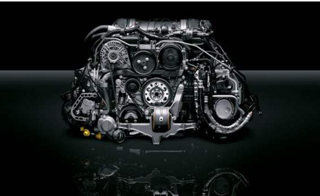
3.4-liter flat-six engine of the Cayman S
