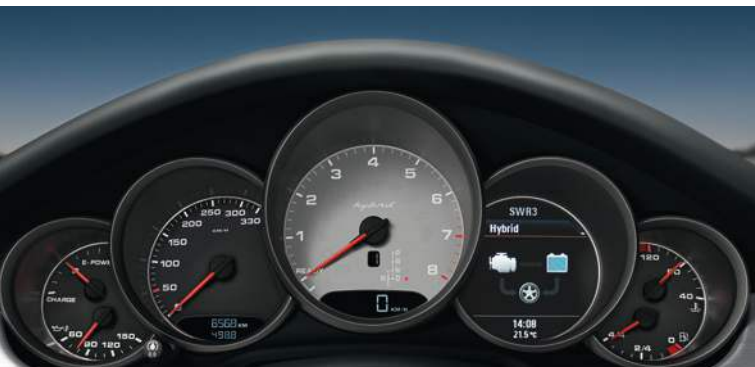
E-Power meter, READY indicator, TFT display in the instrument cluster
