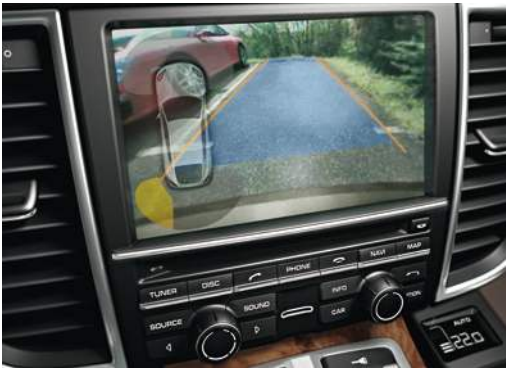
Image from reversing camera in PCM
