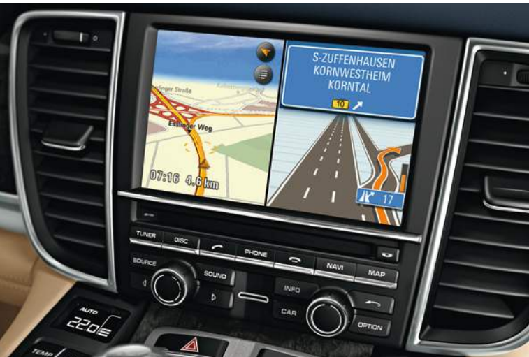
Porsche Communication Management (PCM) with navigation module
