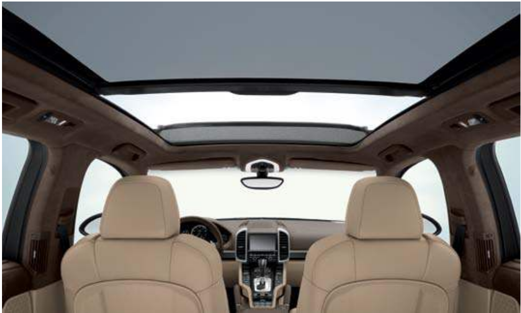
Panoramic roof system
