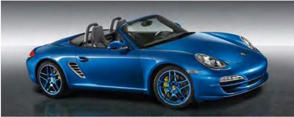
SportDesign package, wheels painted in exterior colour, mirror attachment point finishers painted, exterior mirror lower trims in matt Aluminium Look
