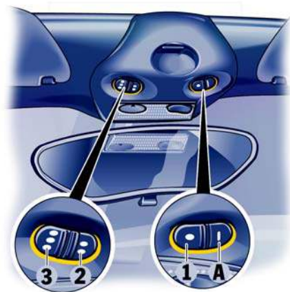
1, 2, 3 - Programmable buttons A - Light-emitting diode for status identification
