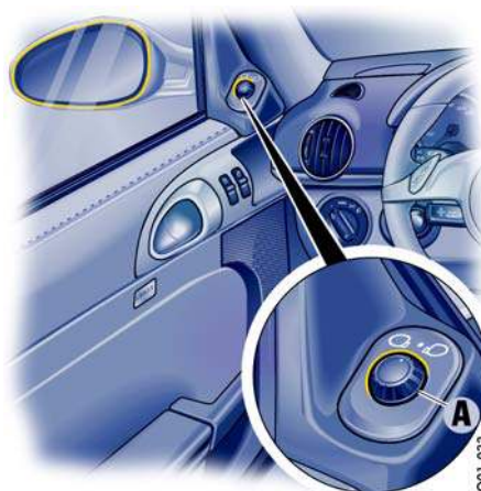
A - Control switch for door mirror adjustment
