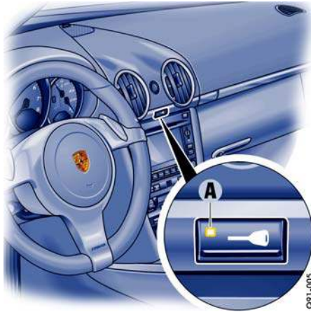
A - Light-emitting diode for alarm system
