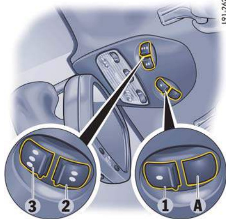
1, 2, 3 - Programmable buttons A - Light-emitting diode for status identification
