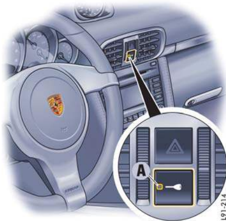
A - Light-emitting diode for alarm system
