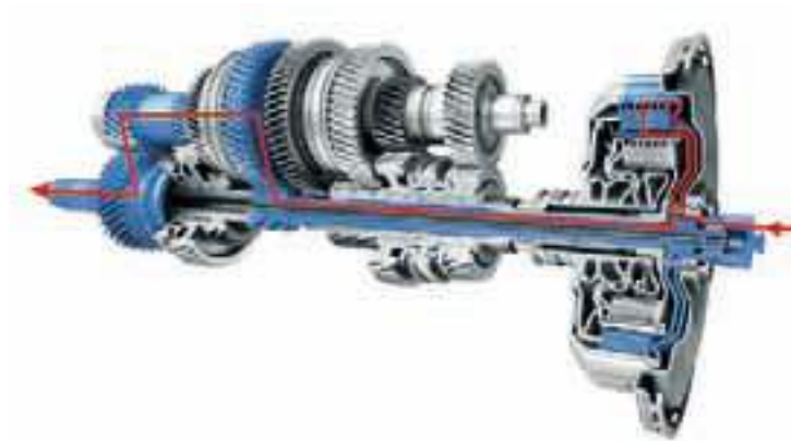
Power flow in 1st gear
