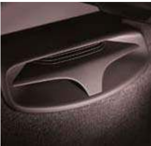
Subwoofer 10.2 cm x 15.3 cm in a 6-litre bass reflex housing
