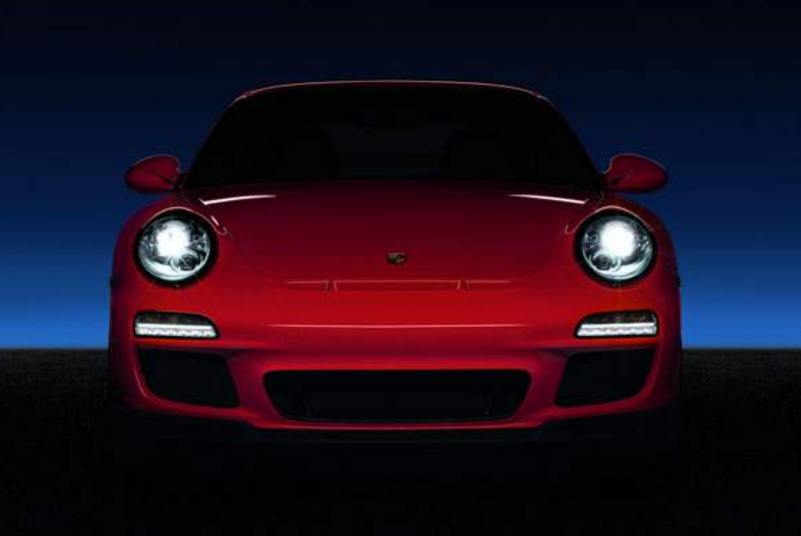
Bi-Xenon headlights and LED position lights
