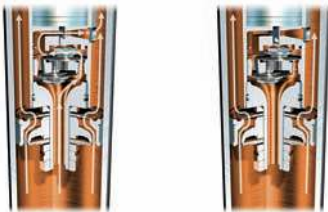
Left: Compression in Normal mode—bypass valve open Right: Compression in Sport mode—bypass valve closed
