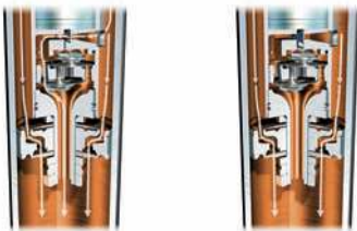
Left: Rebound in Normal mode—bypass valve open Right: Rebound in Sport mode—bypass valve closed
