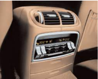
Four-zone air-conditioning system
