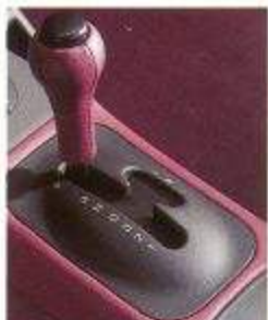
In manual mode, tip the selector forward to shift up, tip back to shift down.
