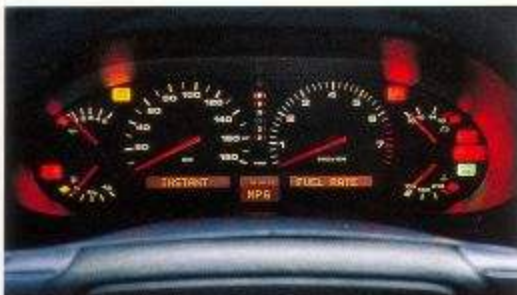
The Porsche 928 GTS's Driver Information Center monitors and prioritizes 22 functions; a flip of a column stalk activates a 10-function onboard computer.
