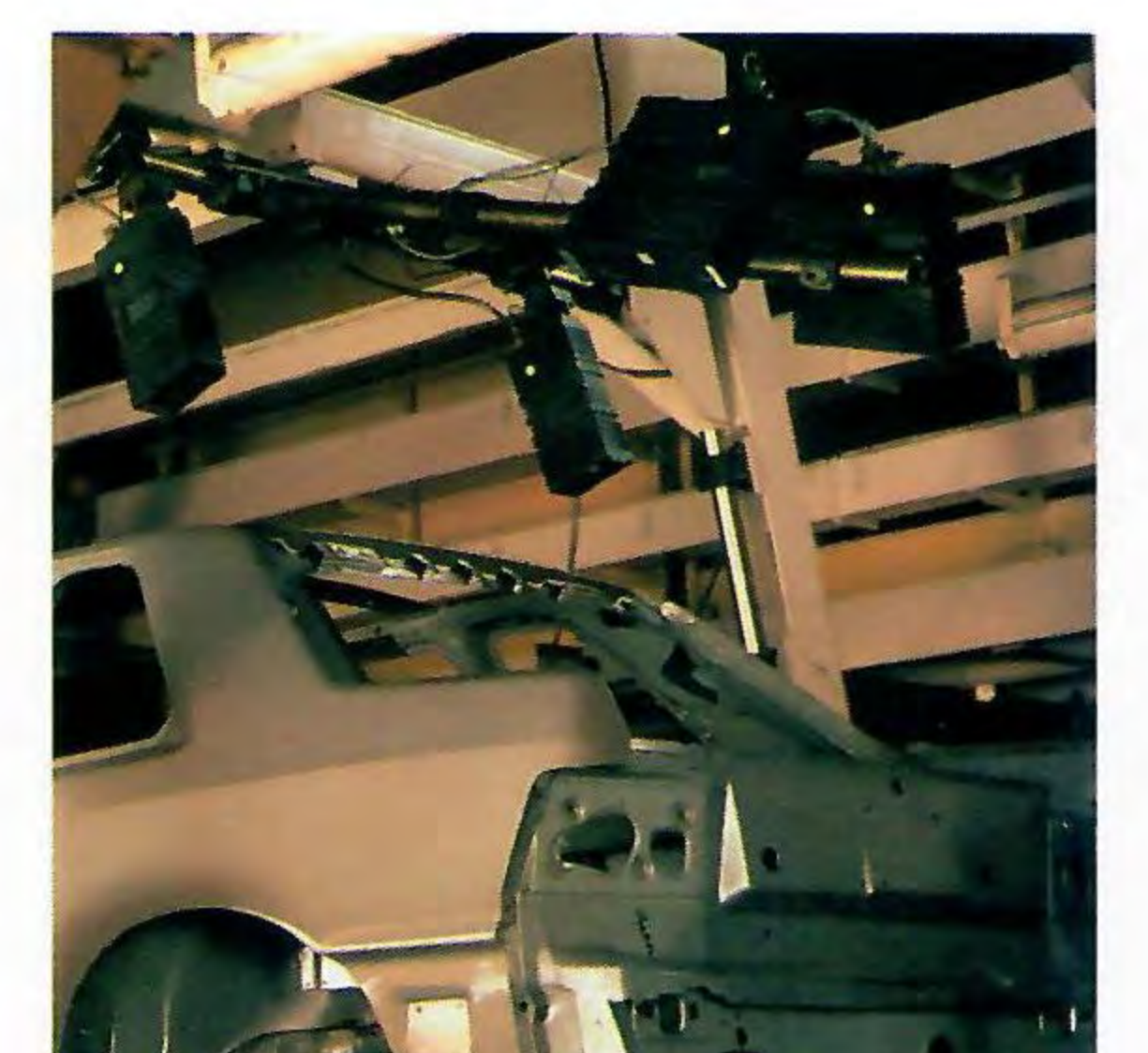
Laser-guided "Mini Perceptron" machine vision system precisely measures body panel fit and finish tolerances to ensure quality.
